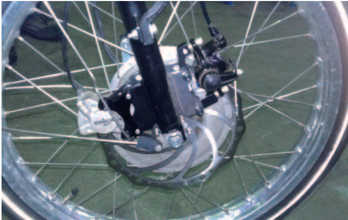
Powerful motor; twin hydraulic disk brakes
